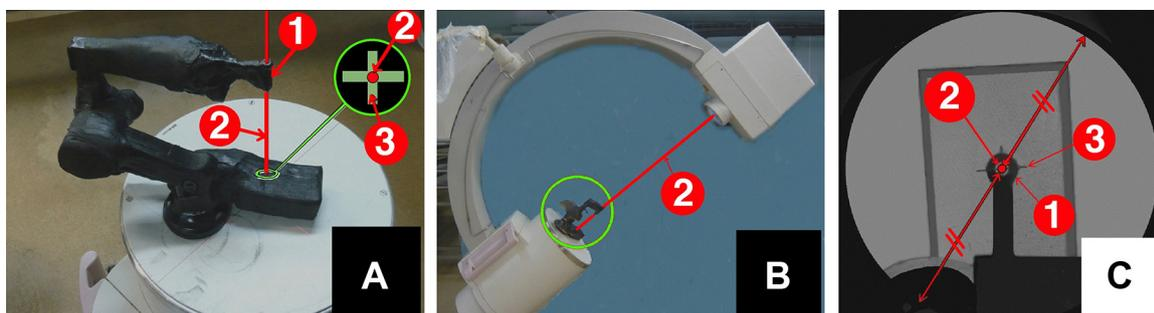
Fig. 3. A–C. Description of the device. The device is attached to the C-arm thanks to a suction pad. The superior part of the open frame is a cylinder (1) while the inferior part is a flat surface bearing a small fluoroscopic cross-shaped marker (3) (A). When properly positioned, the intrinsic axis of the device and the central X-ray beam (2) are aligned (B). Fluoroscopic view showing the alignment of the axis (i.e. the cross-shaped marker appears centered on the projection of the cylinder) (C).
